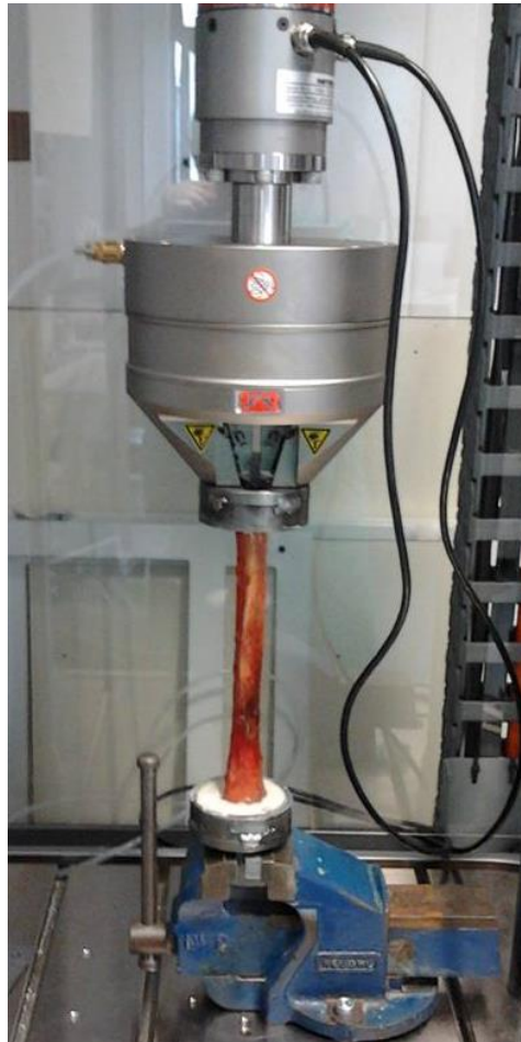
Figure 21: [Experimental set up of a torsion test on the diaphysis of a human tibia using an Instron mechanical testing machine] [taken by Dr Caroline Newe, with permission from the Laboratory of Human Anatomy at the University of Glasgow]
