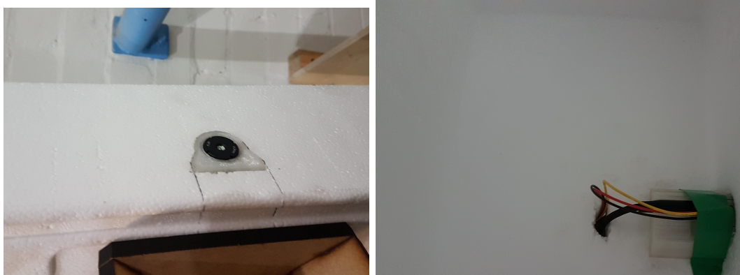
Figure 4.9: Left: FLIR Boson in custom mount enclosed in insulated case; right: external temperature sensor attached to camera housing inside insulated case
