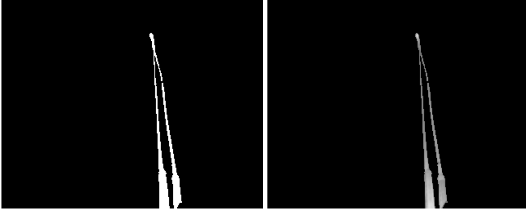
Figure 3.12: Left: Binary region of interest mask; Right: Thermal image of overhead lines with binary mask applied
