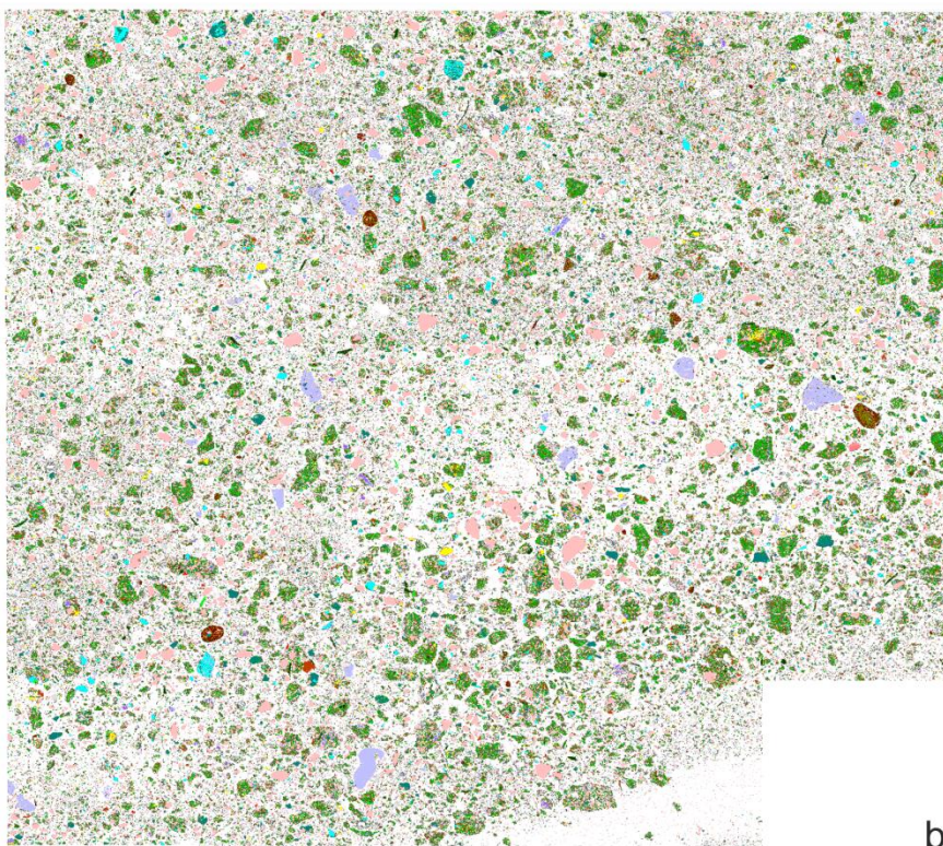
Figure 6.3: a) BSE map of polished section from drill cuttings of mudstone particles from a depth of 700 m in well 4/4-1 and b) false colour map of the same polished thin section showing a mineralogical map and the distribution of main mineral species with Quartz in pink, Illite in green and Pyrite in yellow.
