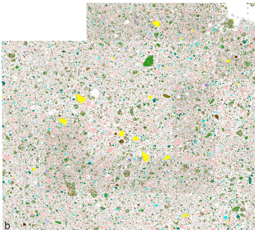
Figure 6.6: a) BSE map of polished section from drill cuttings of mudstone particles from a depth of 850 m in well 4/4-1 and b) false colour map of the same polished thin section showing a mineralogical map and the distribution of main mineral species with Quartz in pink, Illite in green and Pyrite in yellow.
