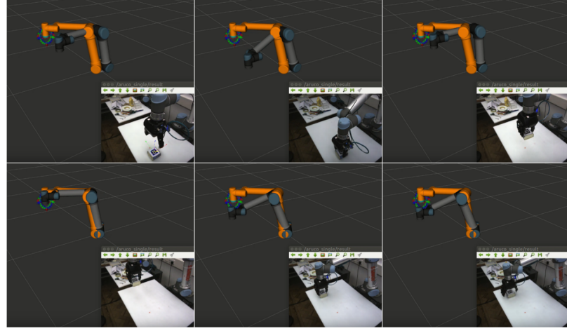
Figure 3.3: Pick and place tasks via the standard path planning method. The UR5 robot arm with orange colour denotes the initial position of the actual UR5 robot arm. The UR5 robot arm with grey colour represents the current position of the actual UR5 robot arm. The image viewer at the bottom right corner represents the view from the 3D camera. The location of the box can be computed by the aruco marker [1] on top of it.
