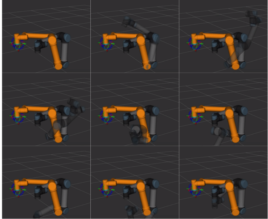
Figure 3.6: Failed path planning with the standard path planning method. The orange UR5 robot arm stands for the initial position of the actual UR5 robot arm, the grey UR5 robot arm stands for the current position of the actual UR5 robot arm, and the transparent UR5 robot arm denotes the planned trajectory for the actual movement of the real UR5 robot arm generated by OMPL in rviz.
