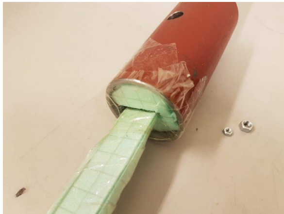
Figure 4.19: Sealing of gaps to avoid grout infiltration
