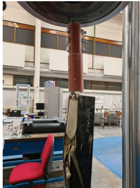
Figure 4.32: Locking of CHS tubes and casing failure under compression
