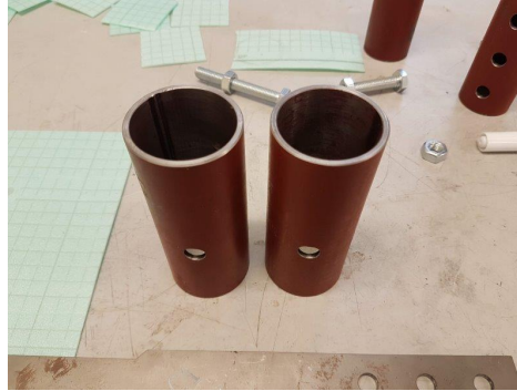
Figure 4.15: Circular hollow-core sections (CHS) used for the connection
