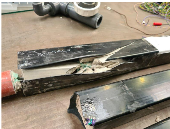
Figure 4.33: Failure of PVC casing of specimen C3
