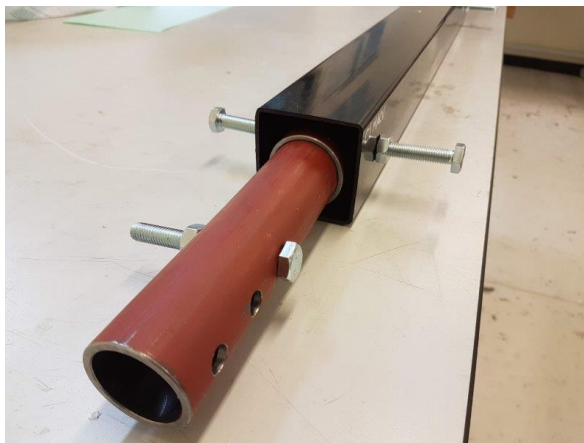
Figure 4.11: Assembly of the manufactured parts. M10 bolts used to centre and position the parts in place
