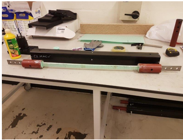
Figure 4.18: Ready parts before final assembly and preparation for grouting
