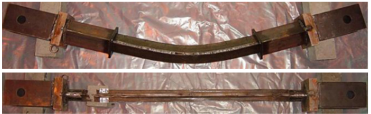
Figure 2.12: (a) 2 point contact mechanism and (b) failed specimen with collar ends from Zhao, B. Wu, and Ou (2012) and Zhao, B. Wu, and Ou (2013)
