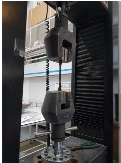
Figure 4.1: Testing of PVC samples
