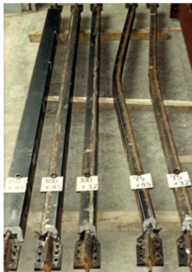
Figure 2.15: Tested specimens from (Watanabe et al. 1988) in (Wada and Nakashima 2004)
