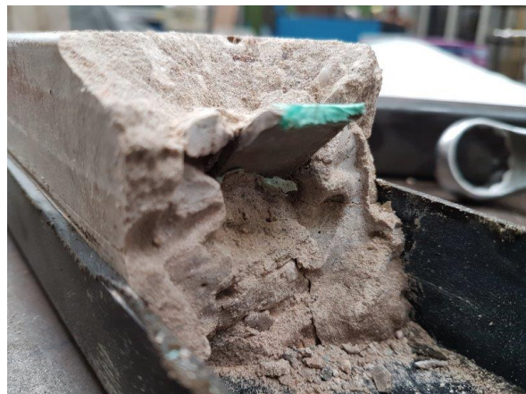
Figure 4.30: Final lateral core displacement in grout punched pocket
