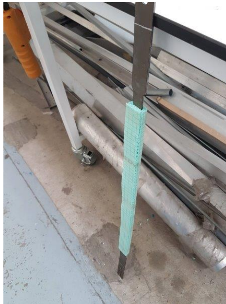
Figure 4.13: Debonding material (extruded polystyrene) applied around the core in layers of 2mm each
