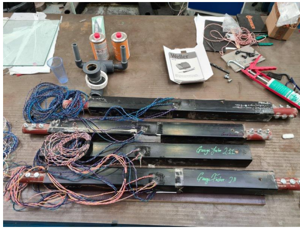
Figure 4.31: Instrumentation of remaining specimens C2, C3 and C4
