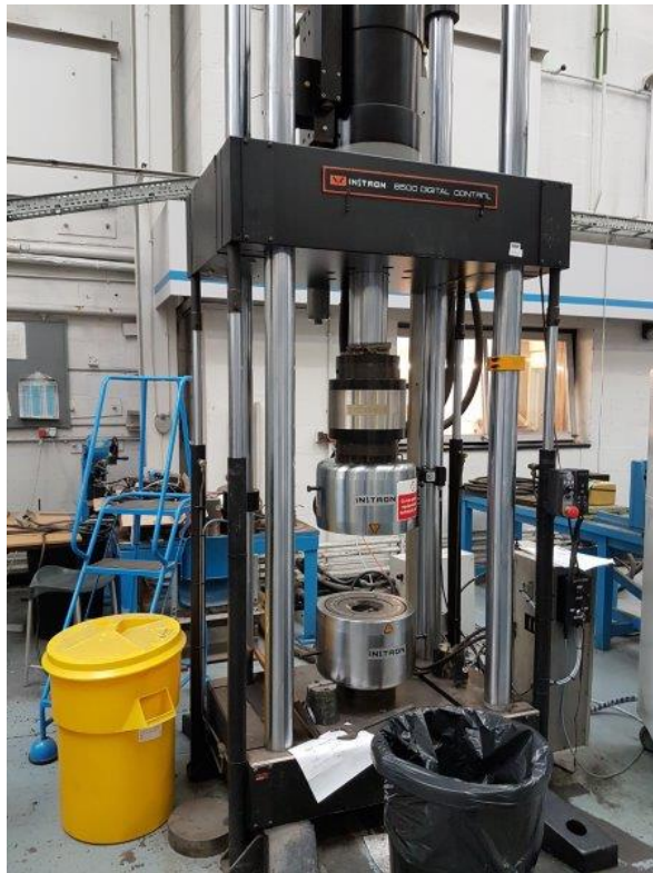
Figure 4.7: Instron equipment for cyclic uniaxial testing with a capacity of 500KN
