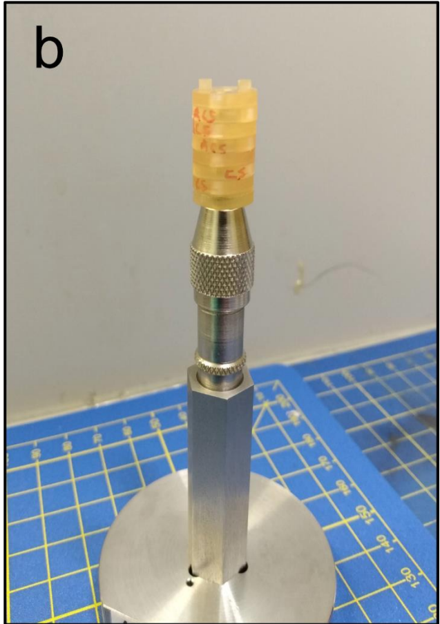
Figure S3. 2. (a) CAD drawing for 3D-printed chuck piece; (b) Photograph of assembled jig clamped in chuck of X-ray CT sample holder; (c) CAD drawing for 3D-printed sample disc holder
