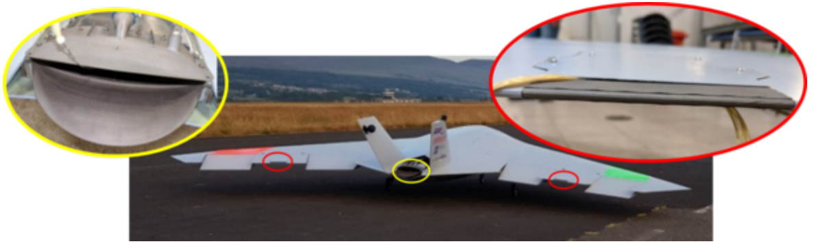
Figure 1.5. Circulation control (yellow) and fluidic thrust vectoring on the MAGMA airframe
