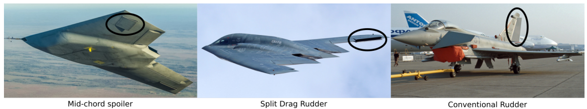
Figure 1.3. Conventional directional control methods 3
