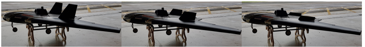
Figure 1.6. Baboo airframe with 100%, 50% and 25% fin height.
