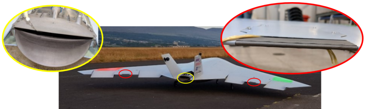
Figure 9.2. Existing fluidic control on MAGMA aircraft.
