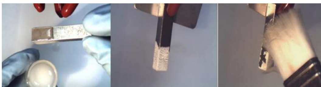
Figure 6- Decontamination by gel immersion followed by mechanical removal (taken from Castellani et al) 42
