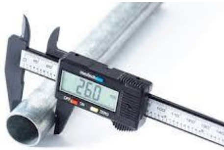
Figure 5-13 Digital vernier caliper for measuring pipe diameter
