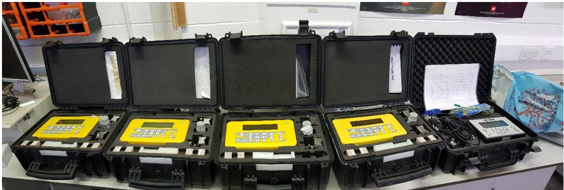
Figure 5-7 PF330 Flowmeters provided by Heriot-Watt University
