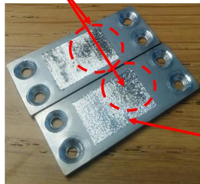
Figure 28 - Examples of printed layers containing localised discrepancies associated with system levelling and discontinuity in the focal plane of the laser. Highlighted areas feature discoloration and poor layer formation.
