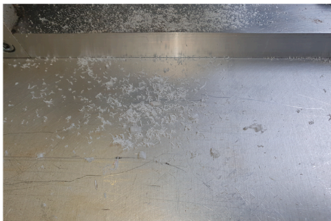
Fig. 23. Coarse debris produced by 22 °C gears at 4 Nm.
