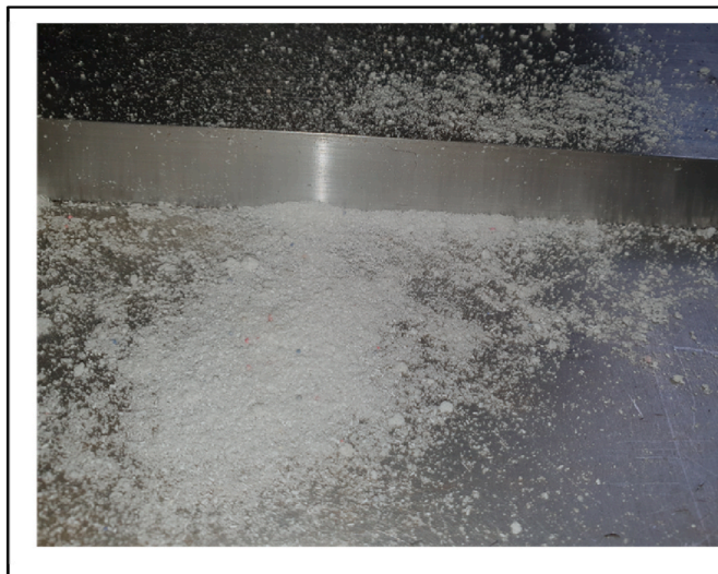
Fig. 20. Fine debris produced by 65 °C produced gears at 0.5 Nm.
