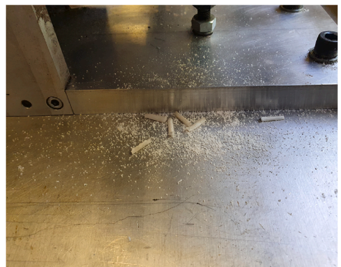
Fig. 21. Mixed debris produced by 65 °C produced gear at 4 Nm.
