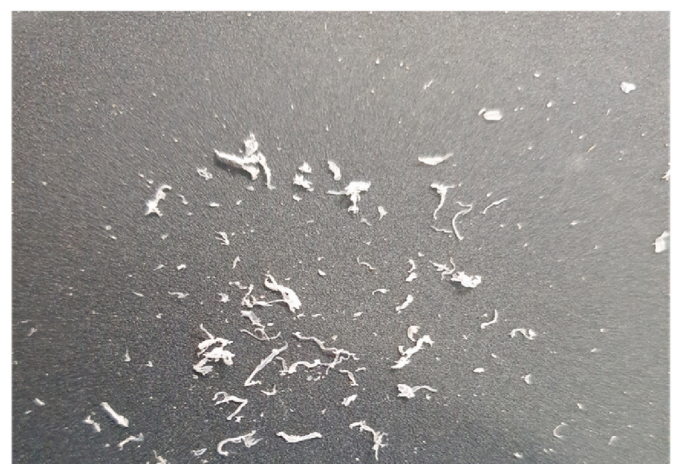
Fig. 22. Coarse debris produced by 22 °C gears at 0.5 Nm.
