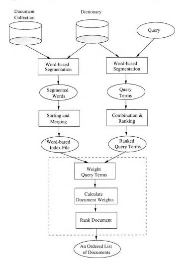
Figure 5.3: System Architecture for Word-based Chinese Retrieval System
