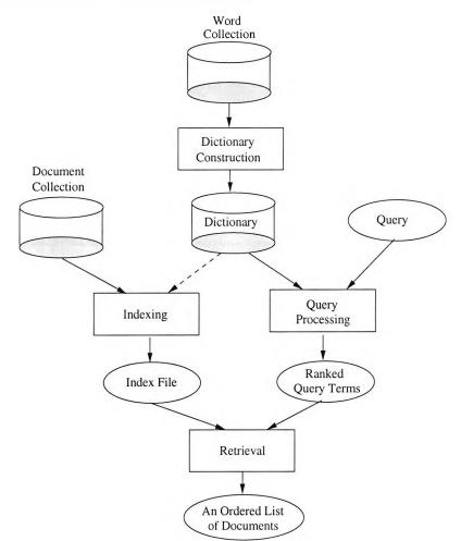
Figure 5.2: System Architecture for Chinese Retrieval System
