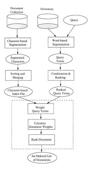
Figure 5.4: System Architecture for Character-based Chinese Retrieval System
