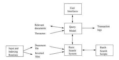
Figure 5.1: Overview of the Structure at Okapi
