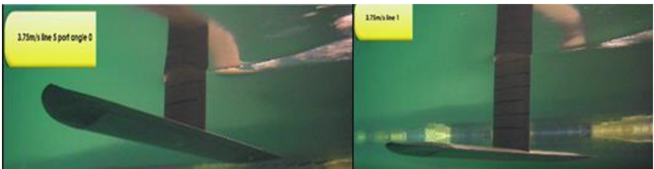
Figure 4. Free surface interaction of unmodified foil at 3.75m/s, 0 degrees – LH 88mm submergence RH 188mm submergence
