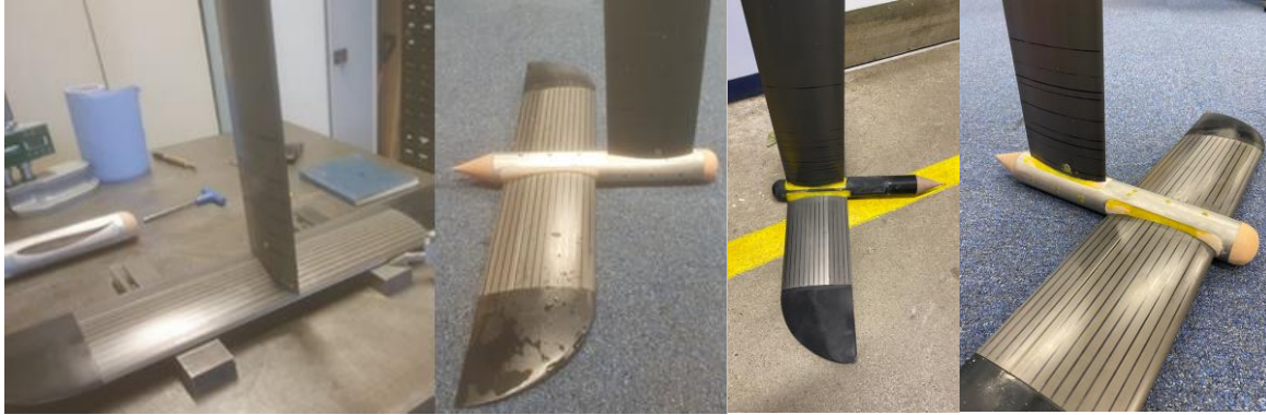
Figure 2. Unmodified foil, foil with horizontal in aft position, foil with bulb, foil with horizontal in forward position
