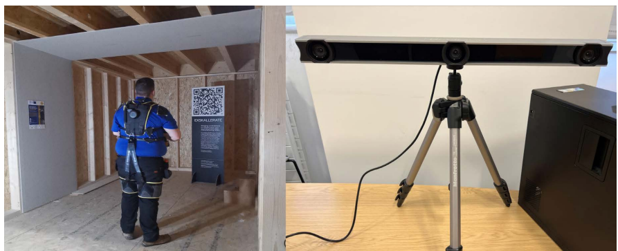
Figure 3. A multiple 3-D point tracking system.
