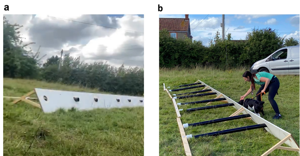
Fig 1. Channelled distance perception rig setup. (a) Channelled distance perception rig setup viewed from the front. For details see text. (b) View of the rig from the back with detection dog Freya and handler Nikki Glover moving along front of the rig checking each pipe entrance.
