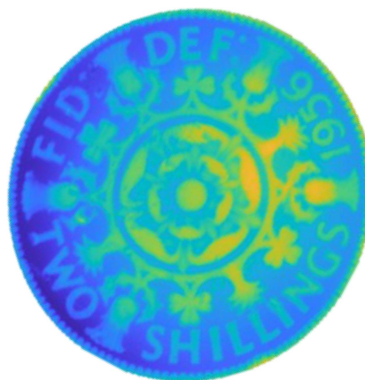
FIGURE 6. Constant frequency scan of the tails side of a U.K. two-shilling coin.
