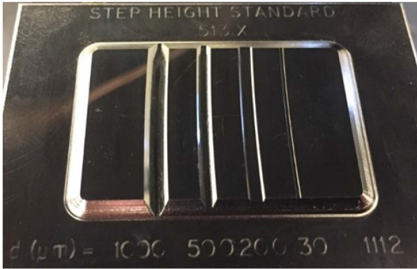
FIGURE 8. A Rubert 513 calibrated specimen formed of Nickel, used as a comparison gauge between measurement modes.
