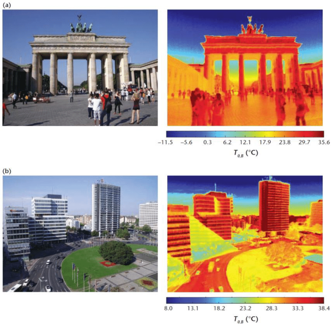
Figure 1.1: Thermal images for two urban landscapes in Berlin, Germany [Oke et al., 2017].
