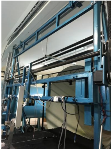
Figure 5-2 Traversing system for the probes positioning into the open test section of the wind tunnel.
