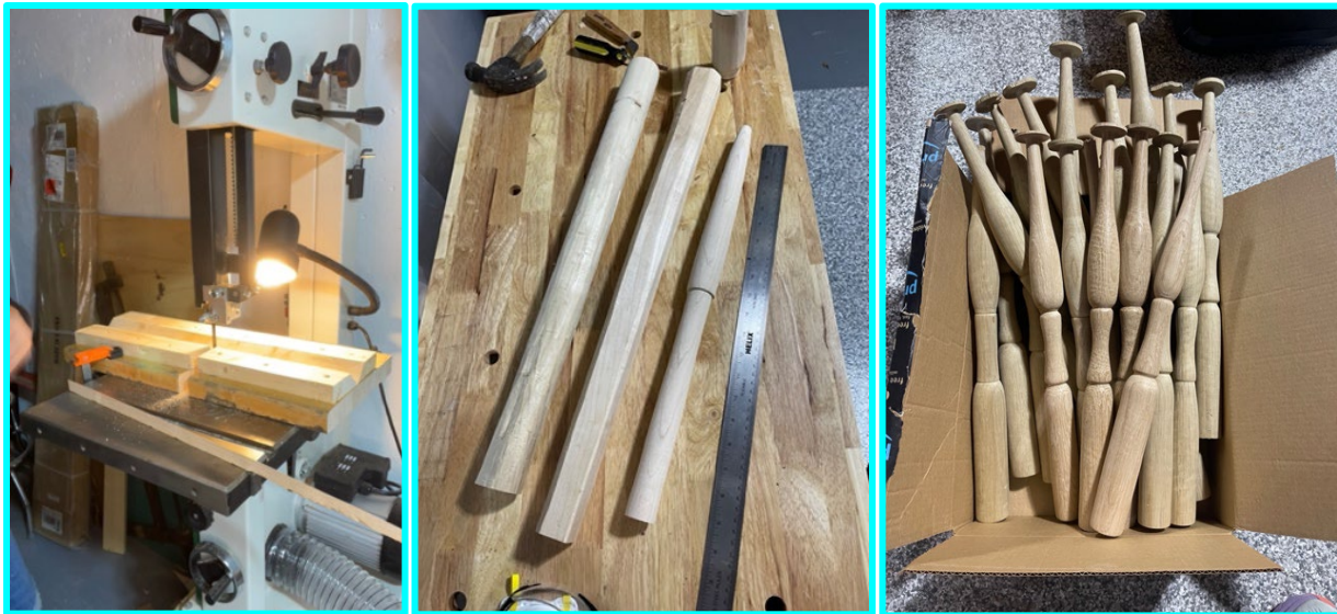
Figure 12. The jig I made for making chair legs (left).
