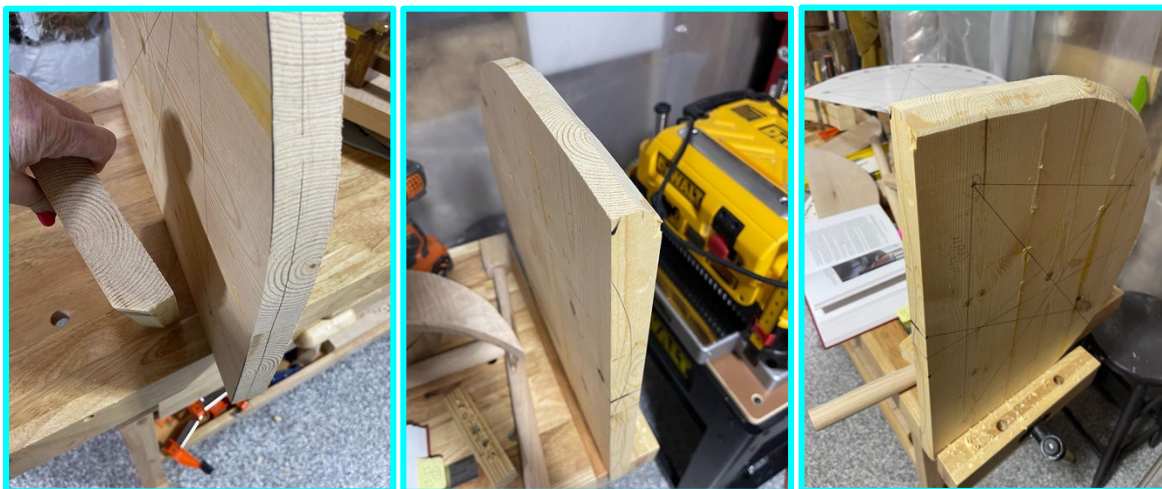
Figure 23. Seat bevel practice and marking (left). Figure 24. Finished practice seat bevel (center). Figure 25. First seat bevel practice on glued practice seat (right).
