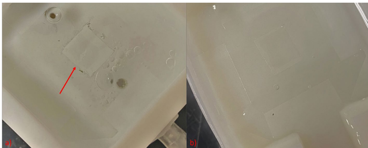
Figure 4.1 a) Broken graphene structure during transfer b) Good quality graphene structure after transfer.
