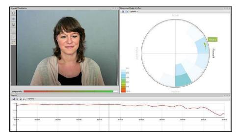
Figure 7.10. Noldus FaceReader Real-Time Expression Analysis Interface. The current frame of motion video shows its coordinate reading of the "happy" label.
