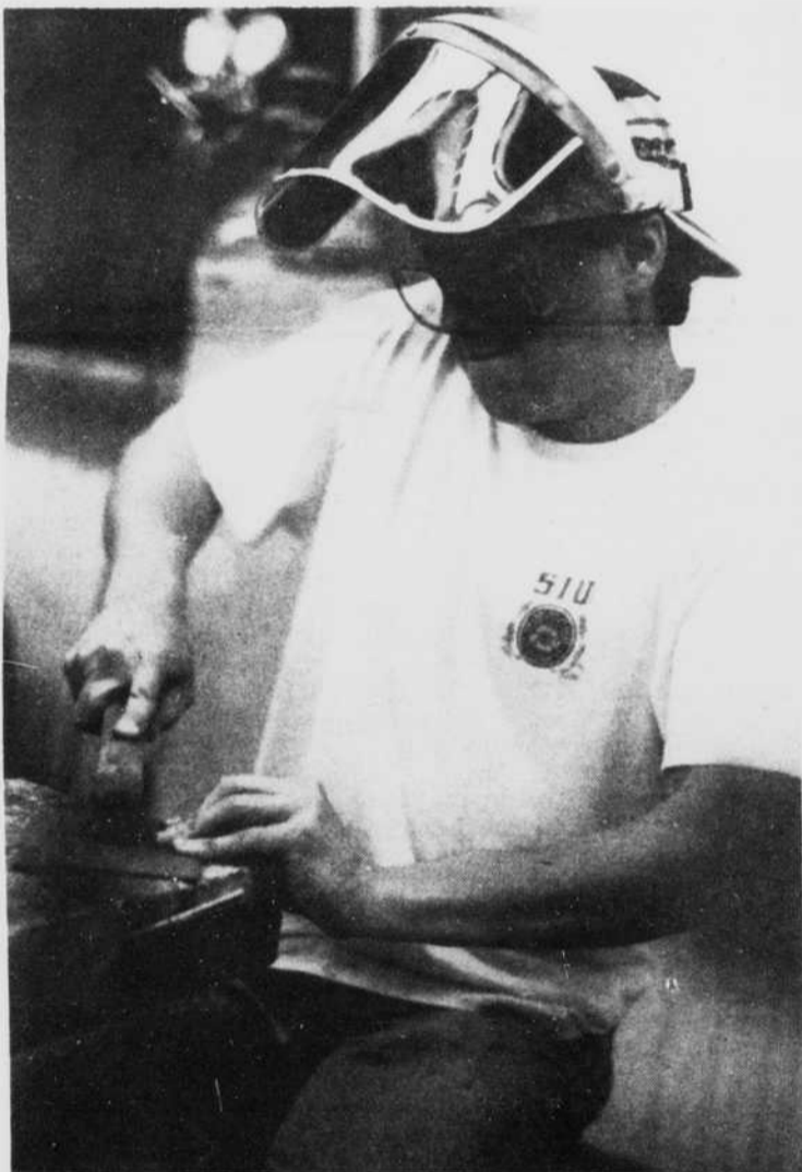
Tony Munzo prepares a piece of carbon steel for welding. The work is done with a wire brush to eliminate surface impurities, thus causing less spattering under extreme heat.
