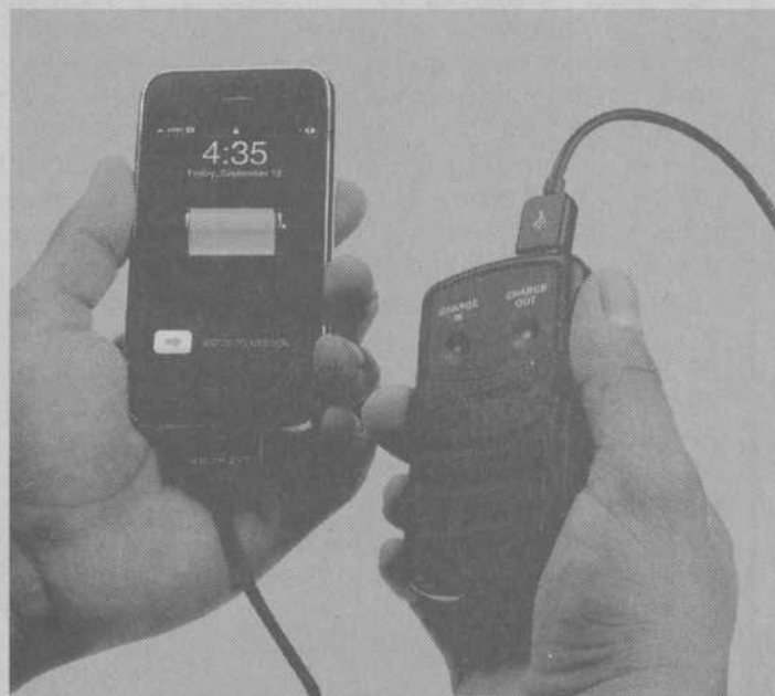
Scosche's solBAT II is a solar powered back up battery and charging device for any portable USB gadget.
