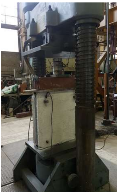
Figure 1a. Insulated composite wall specimen in 1:1 scale [5].
