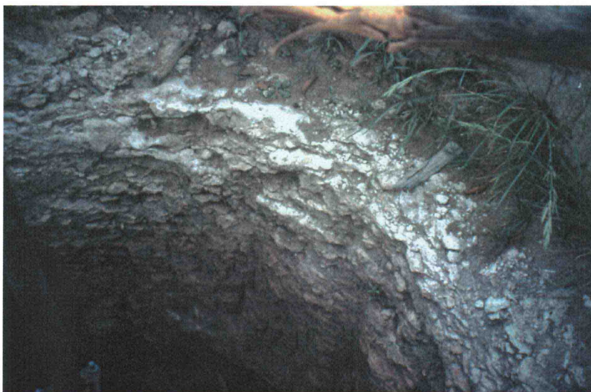
Plate 4.2 Calcrete layer (ca. 50 cm thick; locally known as 'tosca') at ground surface, exposed in a shallow hand-dug well from La Pampa
