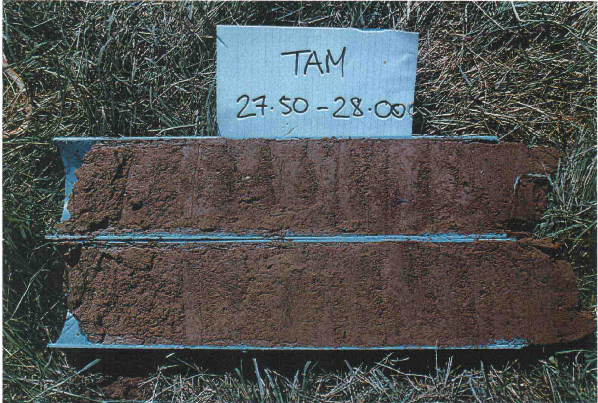
Plate 7.3 Tamagnoni core material (dry brown silt), sample depth: 27.5–28.0 m
