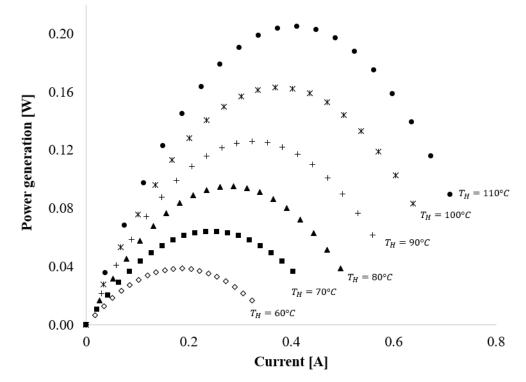
**Figure 2.** Variation of TEG Output Power ( $P_{output}$ ) with Different Hot-Side Temperature Conditions at a Constant Cold-Side Temperature ( $T_{cold} = 24.3 \text{ °C}$ ). Adapted from [25].
