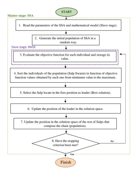
Figure 1. Master-slave methodology proposed SSA/RMSE.
