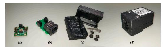
Figure 2. (a) ADXL355 accelerometer (b) adaptor board (c) 3D printed box (d) sensor assembled.
