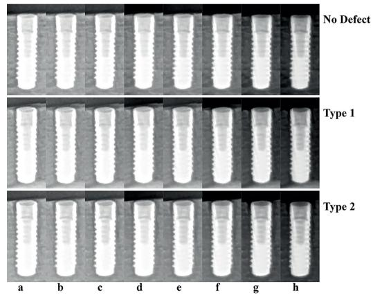
**Fig. 3:** Cropped panoramic images of three different implants in the same bone block obtained with different kV and mA values; (a) 60 kV/3.2 mA; (b) 66 kV/2 mA; (c) 66 kV/3.2 mA; (d) 60 kV/6.3 mA; (e) 72 kV/3.2 mA; (f) 66 kV/6.3 mA; (g) 66 kV/8 mA; (h) 72 kV/6.3 mA.
