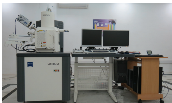
Fig. 3: Field Emission - Scanning Electron Microscope (FE-SEM, SUPRA 55VP).
