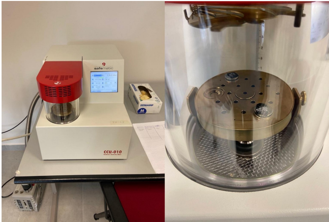
Figure 2.4 (left) Compact Coating Unit-010 (safematic GmbH) for HA particles metallization, (right) HA particles being coated.
