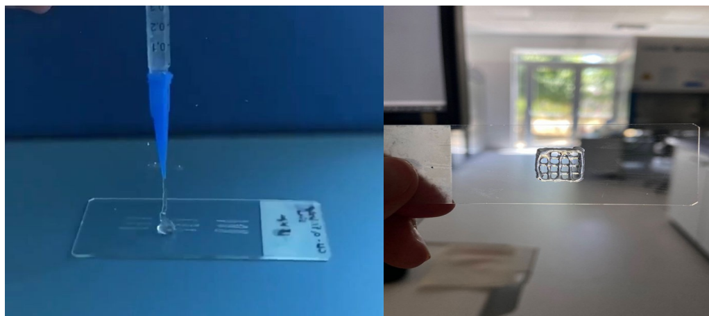
Figure 3.7 (Left) Fiber formation and (Right) example of structure Bioprinted with 0.125% wt/vol SYN_HA.
