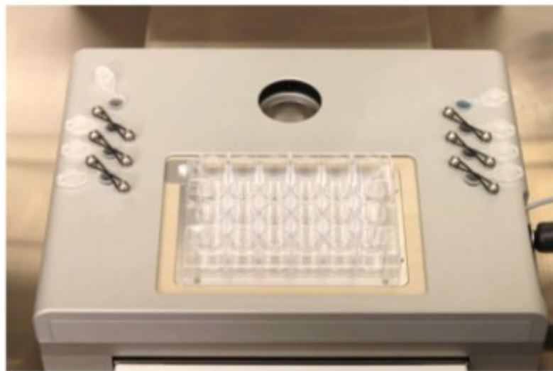
Figure 2.8 Platform cover of Workzone. It's possible to see the cleaning and purging stations, and the workzone where a well plate was fixated.
