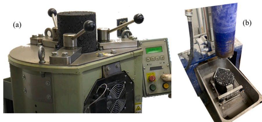
Fig. 3. (a) Gyratory compaction of a 150 mm diameter specimen, (b) extraction of 100 mm diameter cores.
