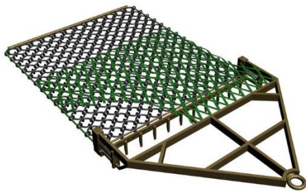
Figure 1: An illustration of a single Newhaven spring-loaded dredge. Image obtained from the Seafish Asset Bank on 11 th March 2022 https://seafish.assetbank-server.com/ .
