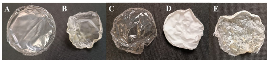
Figure 1. Prepared membranes. (A): CHT, (B): CHT + LEO, (C): ALG, (D): ALG + LEO, (E): CHT/ALG + LEO.
