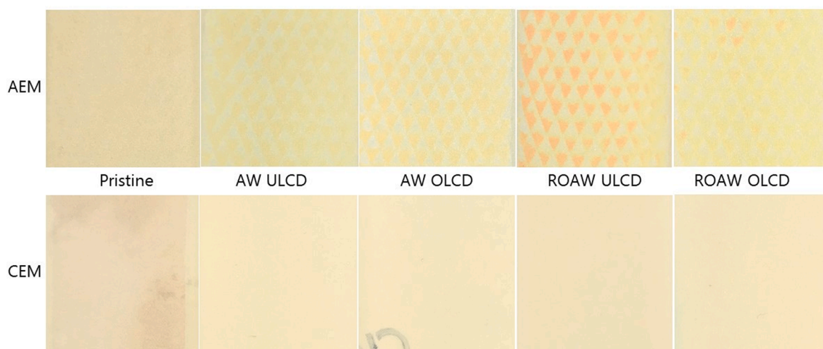
Fig. 4. Photos of pristine and acid whey (AW) and RO pre-processed acid whey (ROAW) fouled AEM and CEM side facing the diluate using underlimiting current density (ULCD) or overlimiting current density (OLCD).
