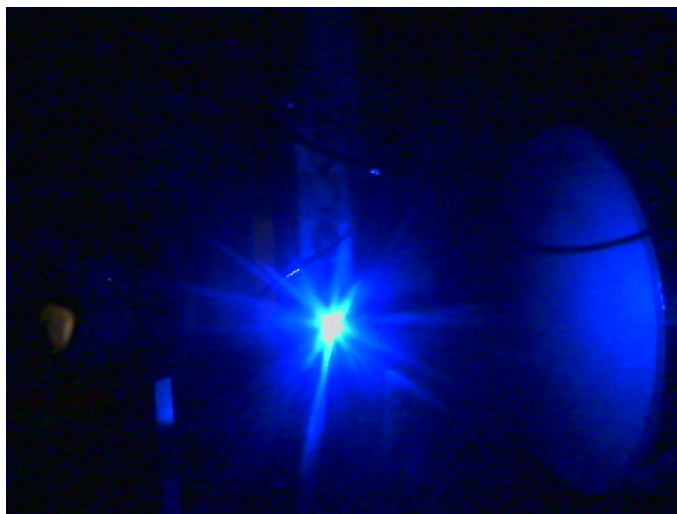
Figure 4.6: Fluorescence induced by a 25 nA beam current.
