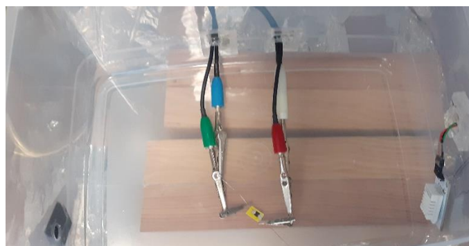
Figure 24 - Inner view of the chamber of the experimental setup of the humidity measurements.
