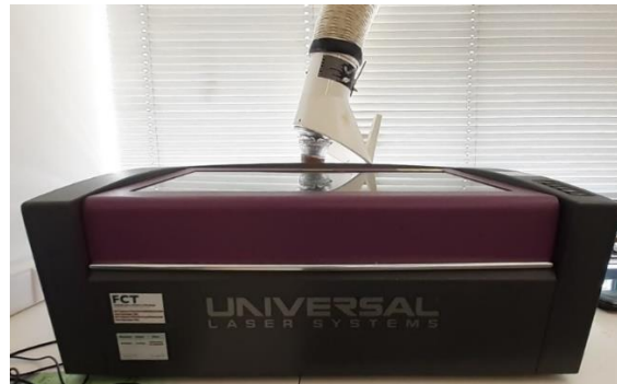
Figure 9 - Universal Laser Systems VLS 3.50 CO 2 commercial at CENIMAT|i3N
