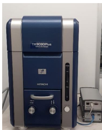
Figure 15 - Hitachi TM 3030Plus Tabletop Microscope available at CENIMAT|i3N
