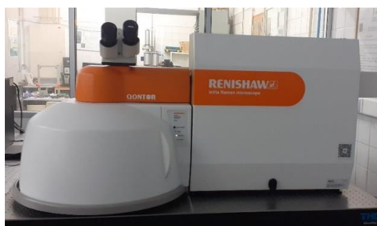
Figure 16- Renishaw in Via Qontor Raman Microscope used in this dissertation available at CENIMAT|i3N
