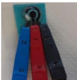
Figure 26 - Demonstration of the final step of electropolymerization WE final step on the pH sensor
