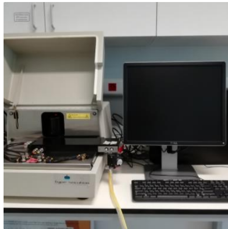
Figure 13 -Biorad HL 5500 sheet resistance equipment at CEMOP laboratory of Electrical Characterization
