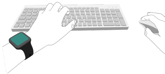
Figure 4.5: Smartwatch placement for data acquisition. Image provided by courtesy of the PrevOccupAI project.
