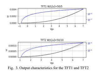
optimization process. Also, since the optimization process is three dimensional and non-convex, bounds to the several parameters had to be considered as a way of obtaining parameter values that are in line with their physical meaning. In the present case  $-2.0 \le V_t \le 1.0$ ,  $10 \le R_s \le 3000$  and  $1.0e - 8 \le K \le 1.0e - 5$  were chosen. Finally, since the output currents to be fitted have very small values, the tolerance was also modified
