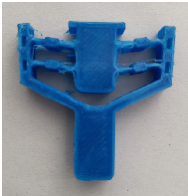
Figure 4.8 — Single cell switching mechanism (after printing).
