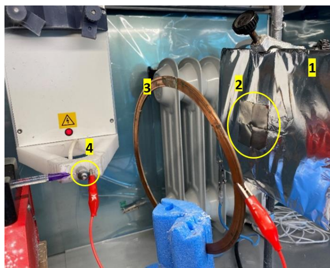
Figure 3.6 - Experimental setup of electrospinning/electrospray collector (1) with four SS substrates (2) attached to it and copper ring (3) attached to the syringe needle (4) by crocodiles.
