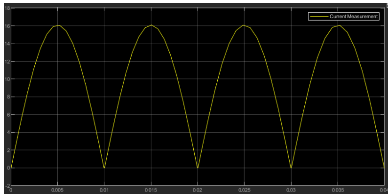
Figure 4.9: Current behaviour of the full-wave bridge rectifier. Vertical axis is current (A), horizontal axis is time (s).
