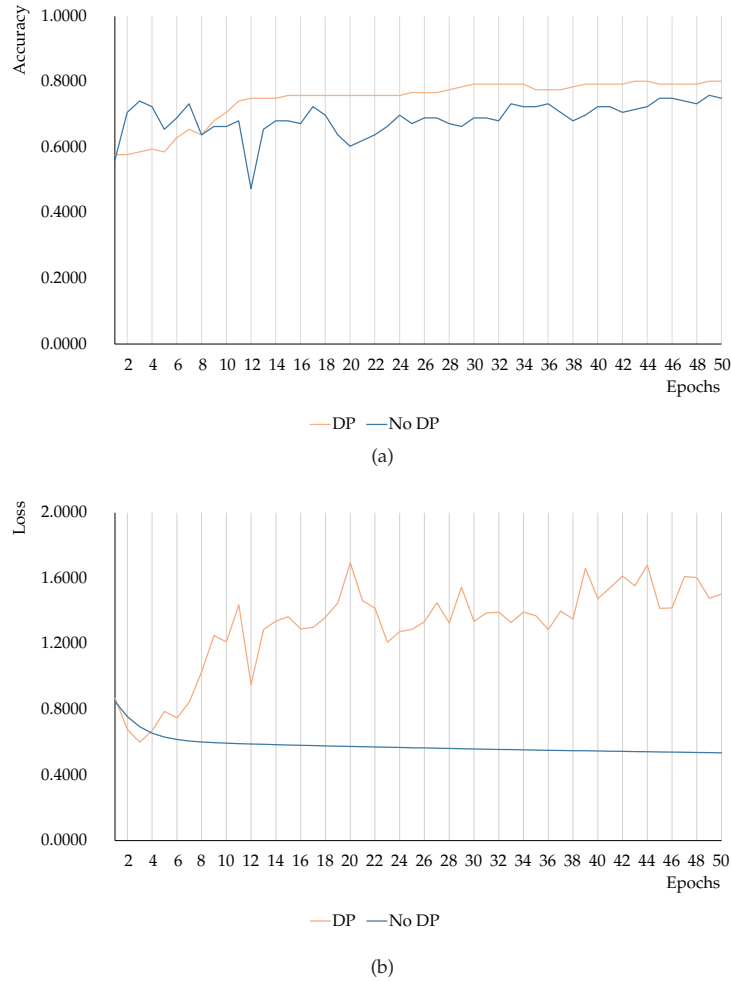
Figure 6.9: Comparison of the training accuracy (a) and loss (b) of the FEDAVG algorithm with fifty global epochs, five local epochs with and without the usage of DP with a noise value of 5.
