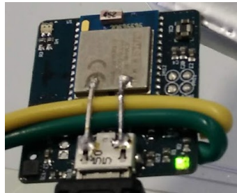
Figure 4.9: Prototype of the data acquisition unit to be embedded in the tablet. The green and yellow wires are alligator clips soldered to the ECG front-end and used to connect the dry electrode samples. The device's PCB footprint is a 2.5 x 2.8cm rectangle.
