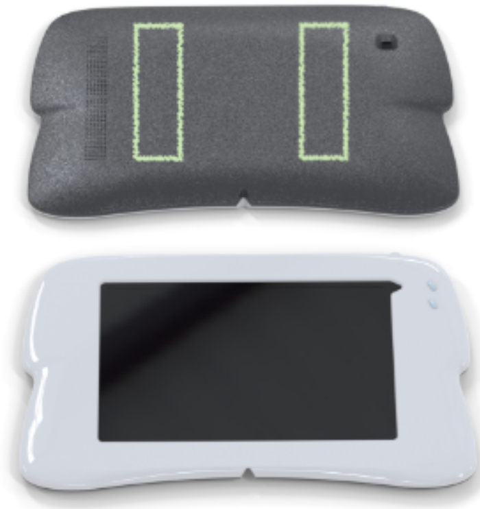
Figure 4.15: Pre-production unit of the final design for the tablet. This unit featured a custom back cover without the electrodes embedded, serving as a visual aid. Thorough tests will be done for optimal electrode placement in the back cover to ensure long-term comfort while using the tablet and recording ECG . In green, a conceptual position for the electrodes.
