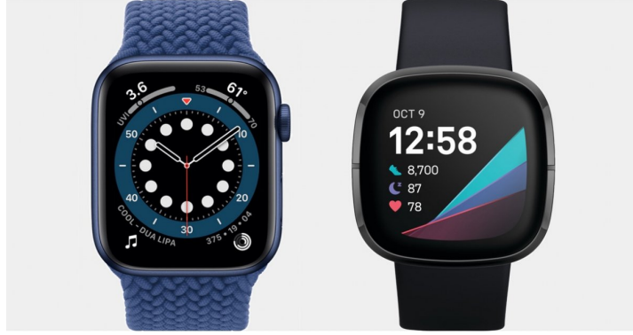
Figure 1.3: Two popular ECG-enabled smartwatches, namely the Apple Watch (left) and the Fitbit Sense (right), capable of recording and processing 30 seconds rhythm strips.
