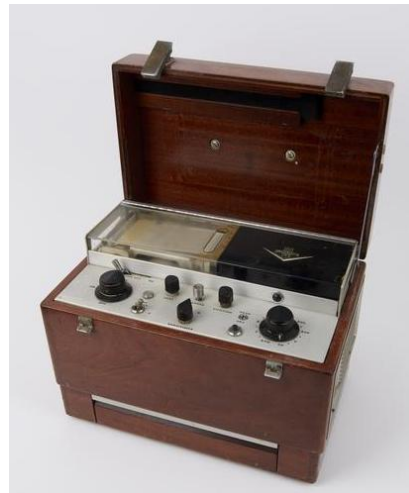
(b) Sanborn Viso 100 portable ECG machine from 1935-1955. Extracted from [43].
