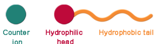
Figure 1.5. Amphiphilic structure of SAILs. Adapted from Buettner et al , 2022 [29].
