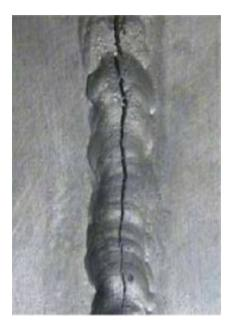
Figure 3. Weld crack adapted from [12].
