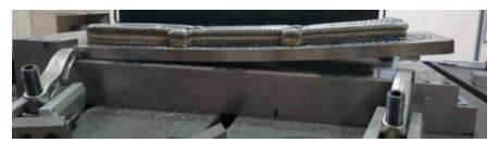
Figure 10. Geometric distortion, adapted from [24].
