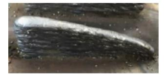
Figure 9. Uneven bead height, adapted from [17].
