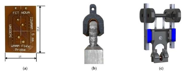
**Figure 22.** Multi-layer flexible PCB probe; (**a**) PCB; (**b**) PCB assembled in the TPU chassis mounted over a WAAM wall specimen; (**c**) complete probe set-up system.
