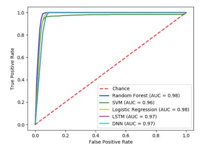
**Fig. 2.** Receiver Operating Characteristic (ROC) curve: performance obtained on the *large* dataset by Random Forest, SVM, Logistic Regression, deep net with lstm layer (LSTM), and deep net with only dense layers (DNN). All the models learned to correctly recognize the items with minor mistakes.
