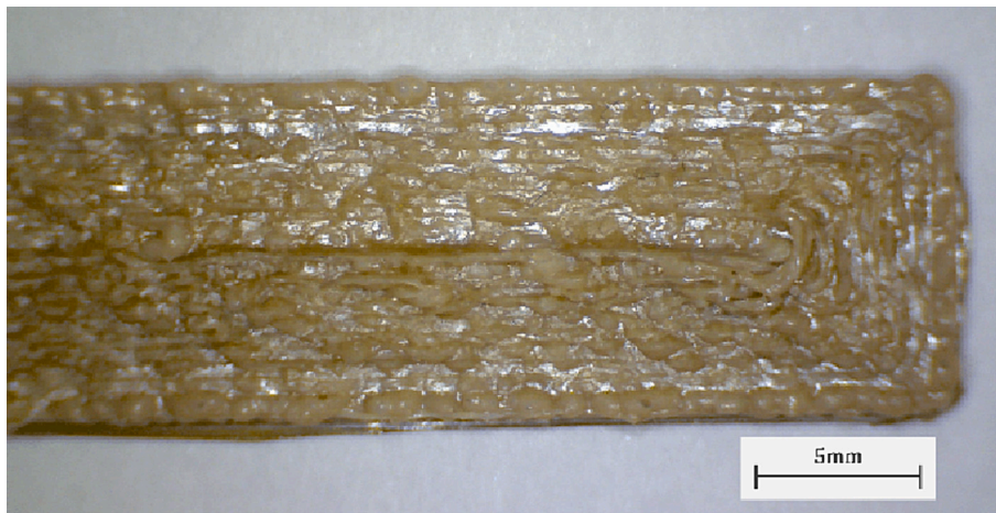
Fig. 11. Surface quality of flexural test specimen C10 printed with an extruder multiplier of 1.1.
