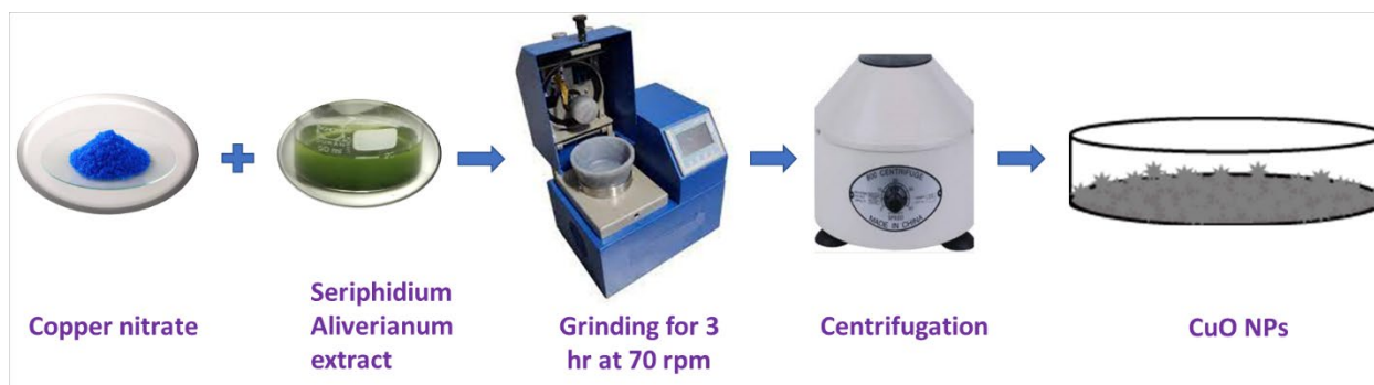
Figure 11. Mechanochemical synthesis of biogenic CuO NPs.
