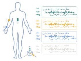
Fig. 2. Schematic of the placement of Inertial sensors, used for the dataset acquisition protocol. Based on [1] and [3]
