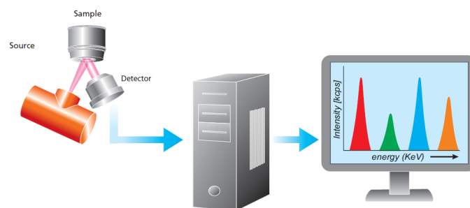
Figure 2.6: Illustration of a typical EDXRF Setup [9]
